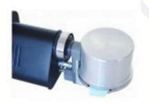
MO-2M collects air samples from inspected objects, either directly or after vaporization explosives traces in TVIN. Vapors are then ionized and separated using the Non Linear Dependence of Ion Mobility (NLDM), also called FAIMS
