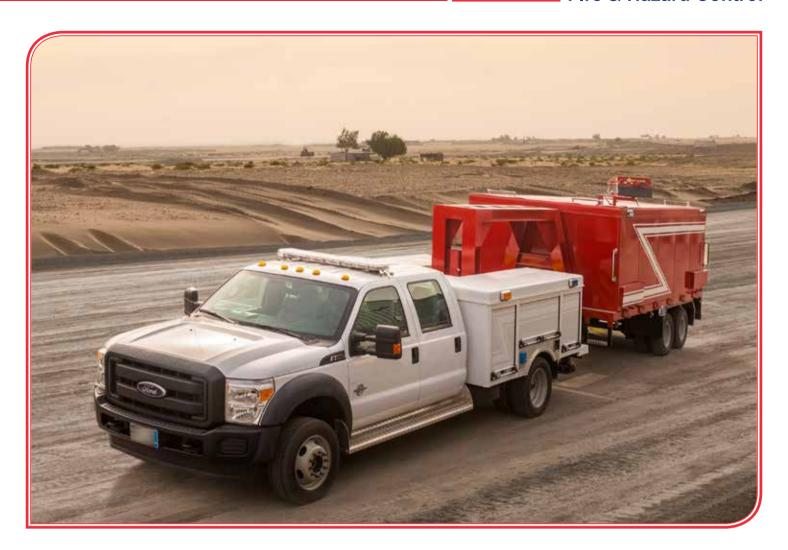
The REDA Fire & Hazard Control engineering team has created a versatile combination using the REDA custom built light rescue body and various trailer units. The chassis mounted equipment body and trailer body are all constructed of aluminum using custom designed extrusions for a corrosion free body. The bodies are available in various lengths to accommodate purchaser's equipment and LDH fire hose inventory.
